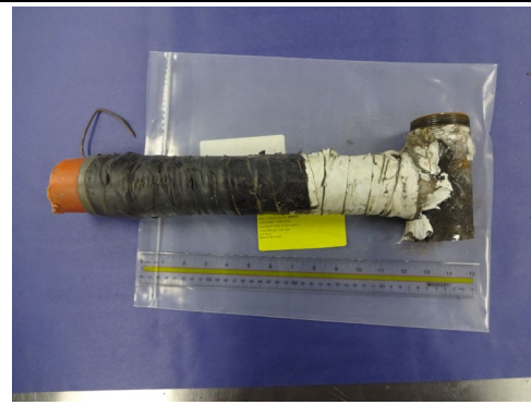
Figure 4. Mueller Tee after removal from scene. 3
