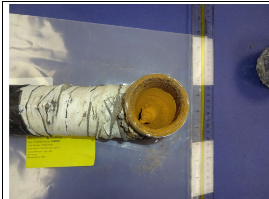
Figure 5. Top view of Mueller Tee showing top of X-Pando Plug. 3
