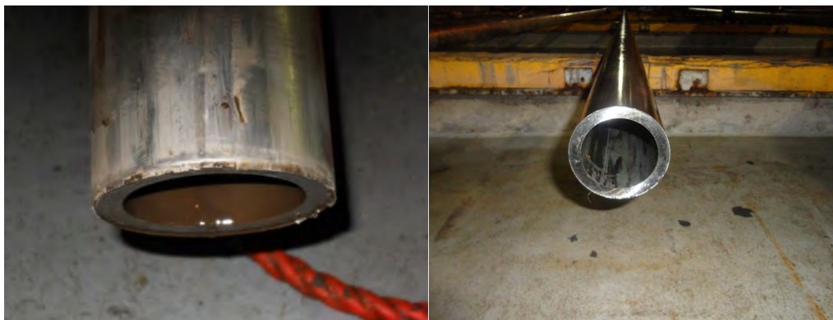
Figure 38. Tubing Cut with the Baker Mechanical Pipe Cutter
