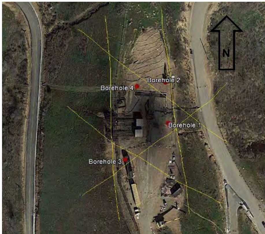
Figure 34. Shallow Borehole Locations
