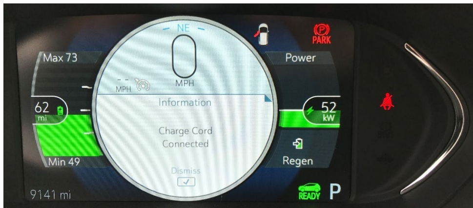
Image 15: Chevy Bolt charging at 52 kW on ABB 175 kW charger from commissioning test.
