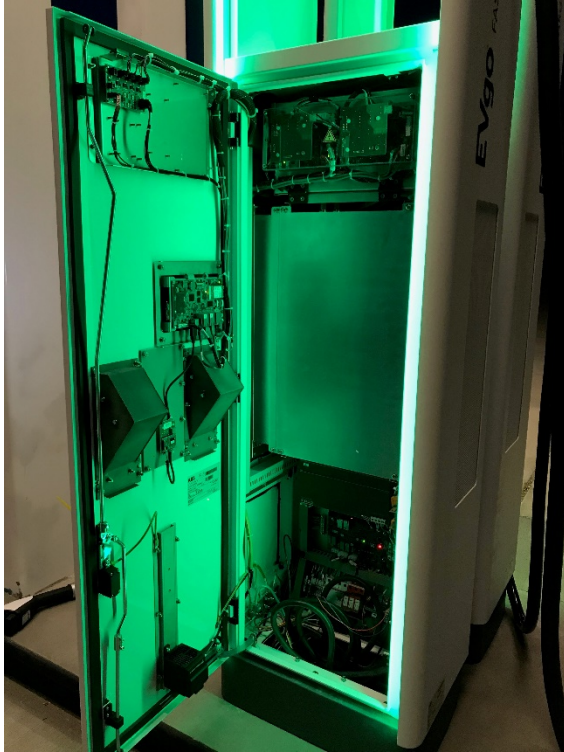
Image 5: ABB charge post interior.
