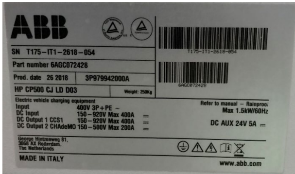
Image 7: ABB charge post nameplate.
