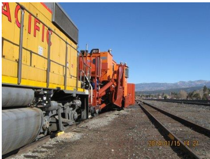
UPRR Truckee Yard, Track #115 looking East --Jordan Spreader fouling adjacent track. The equipment should have been left behind the yellow marker, visible under the locomotive.
