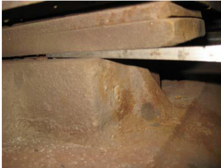
Petroleum tank car with insufficient side bearings clearance UPRR West Colton Yard
