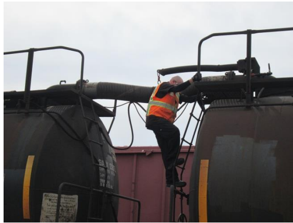
Inspecting typical DOT-111A tank cars on San Ardo to Dolores oil train. Some cars have a built date of 1977. Cars have a life expectancy of 50 years.
