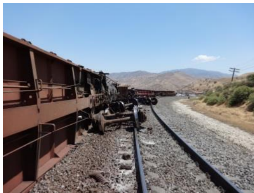
Derailment, Tehachapi Pass, May 5, 2015. This derailment occurred in Local Safety Hazard Site #16, UPRR Mojave subdivision, specifically, at railroad station Caliente. The cause was a broken coupler (rail car connection device).
