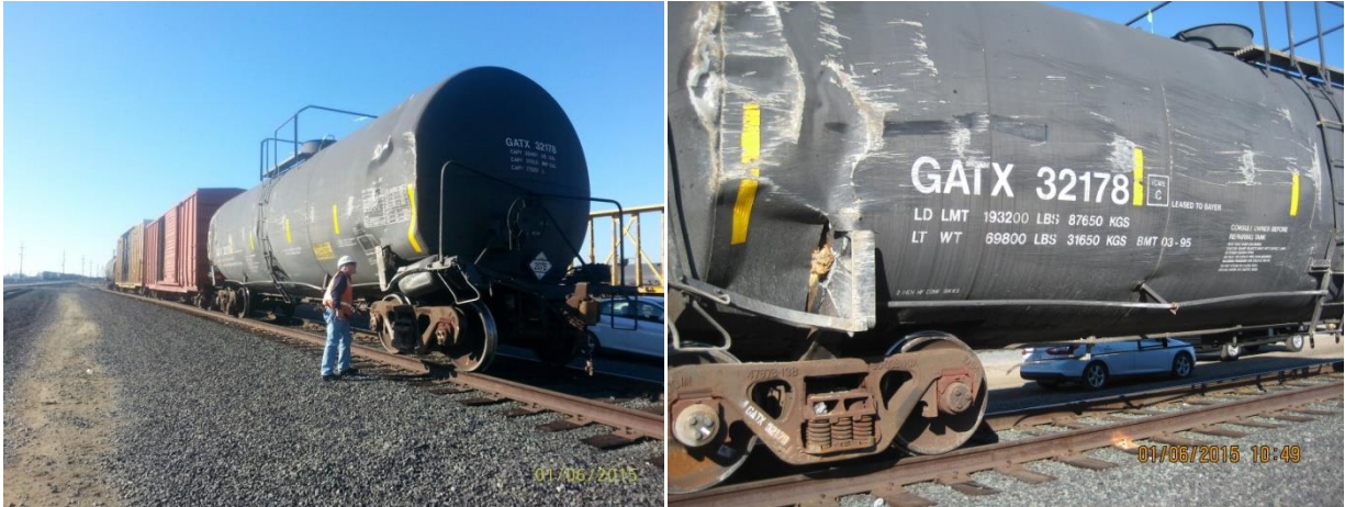
CPUC Railroad Safety Inspector examining damage to a tank car as a result of the derailment
