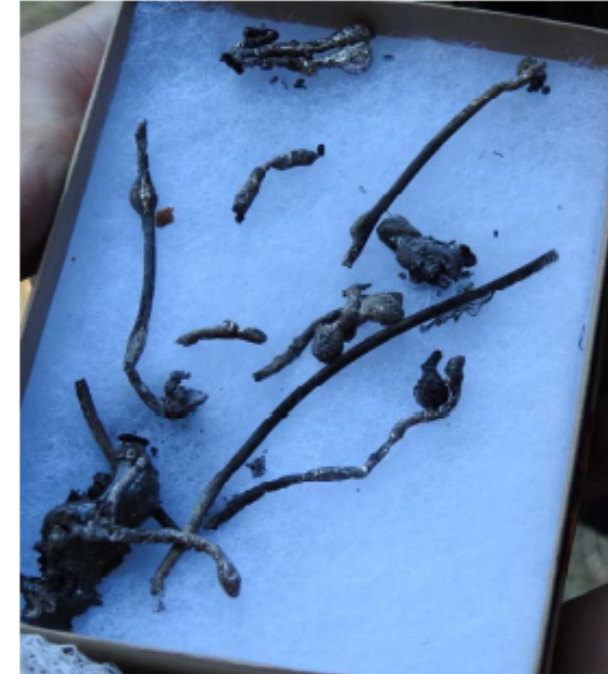
Figure 11. Failed pieces of conductor strands and evidence of arcing.
