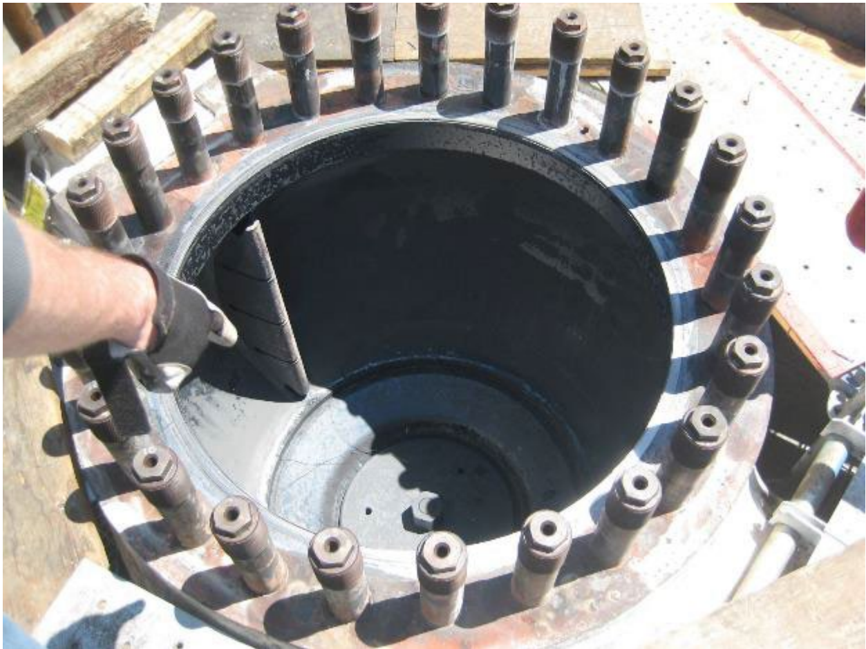
Figure 29. Combined Hot Reheat (CHRH) valve was open for inspection and analysis. A forensic analysis by Structural Integrity Associates indicate this valve played a key role [REDACTED].
