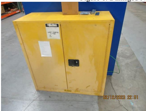
Figure 7 & 8: NFPA Fire diamonds missing on the flammable storage cabinets
