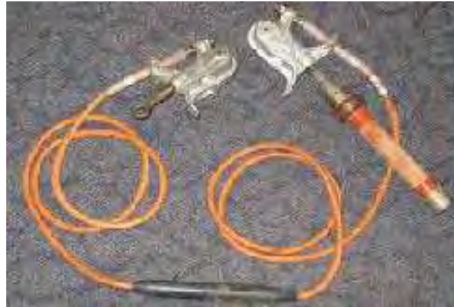
Figure 5-7: Duckbill to Red Head Duckbill Break-away Bond 2/0 Conductor Size
