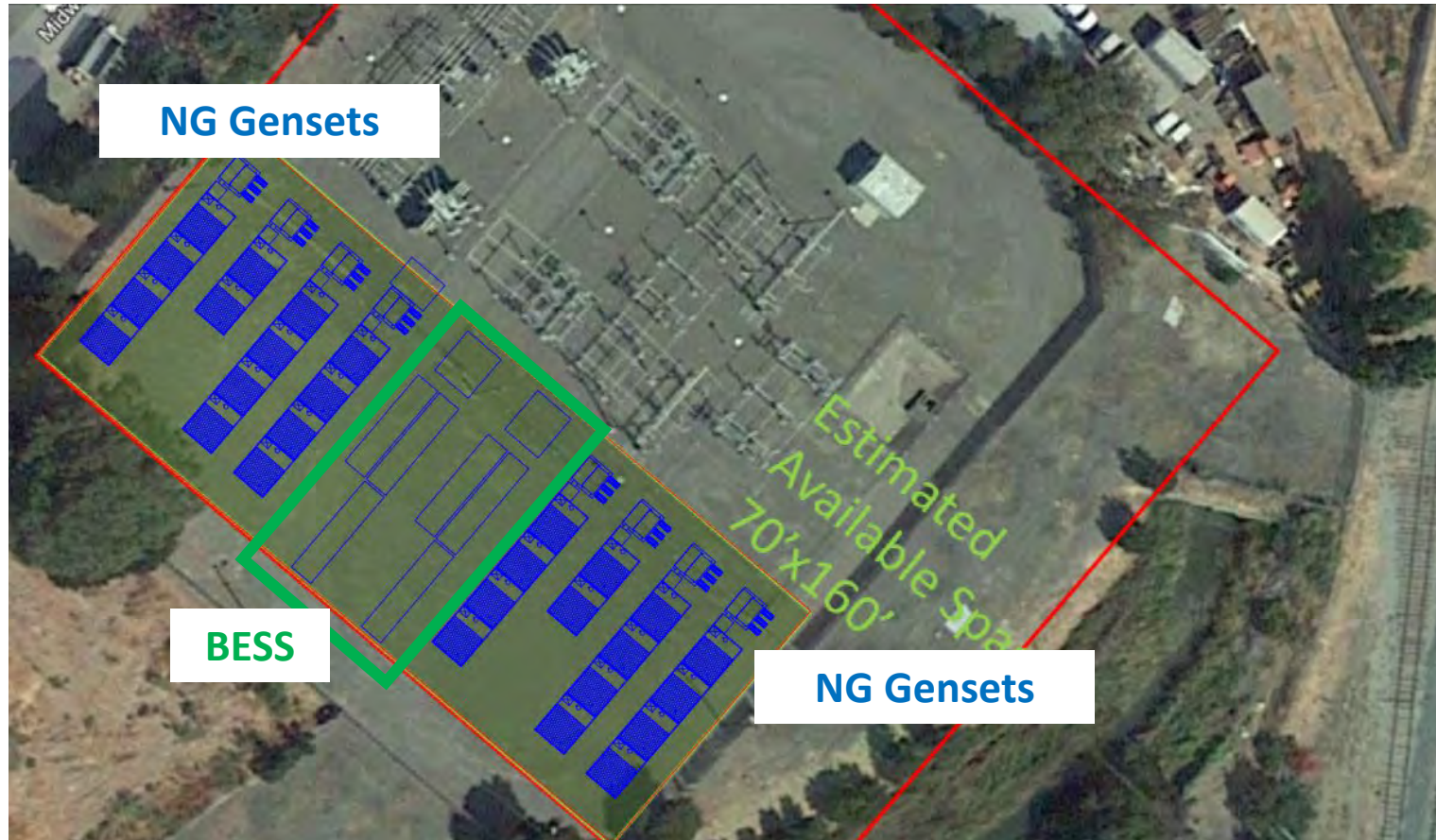
Carquinez Substation – 12.2 MW NG, 4.4 MW BESS Vallejo, CA
