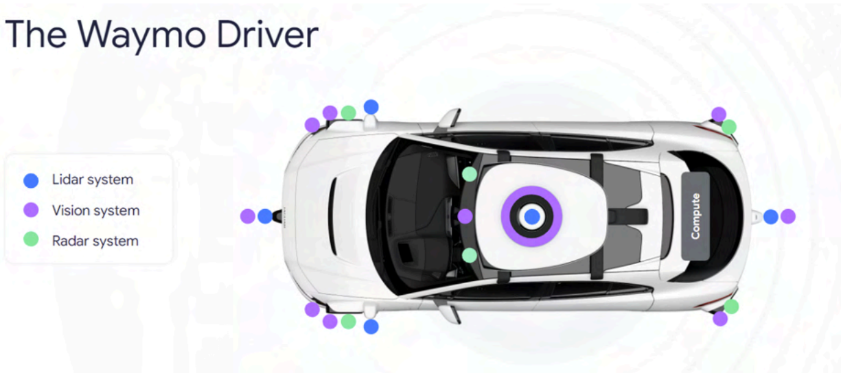
Fig. 1 Illustration of the Waymo Driver sensor suite 3
